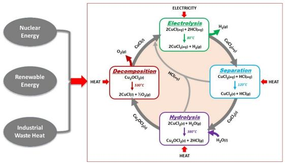
Figure 4. Hybrid Cu-Cl thermochemical hydrogen production
