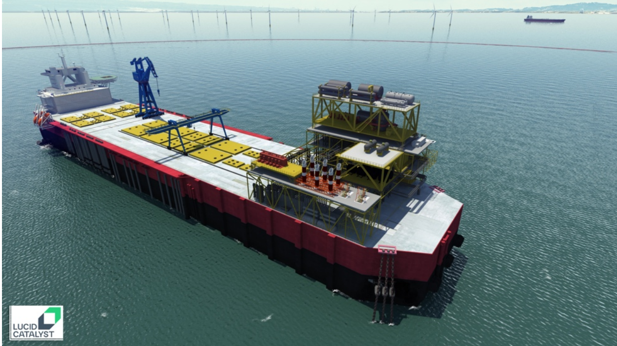
Figure 5. Shipyard-manufactured hydrogen, ammonia, and desalination facility
