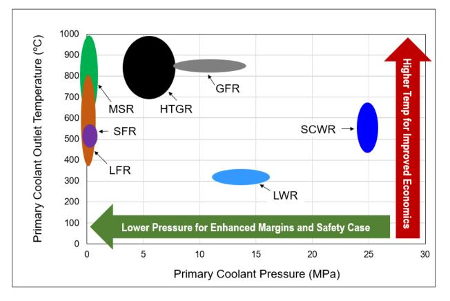
Figure 2 Primary coolant outlet temperature vs. pressure for current and advanced reactors.
