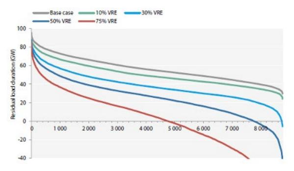
Figure 2. Residual load duration curves at different VRE shares, illustrative cases
